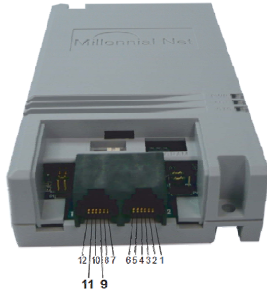
Figure 1: RJ11 Connector Contact Numbers on Wi-IO
